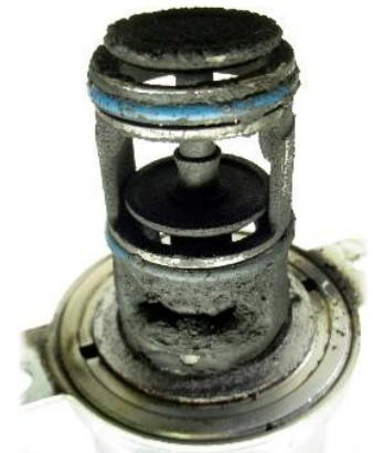
Figure 1: Failed EGR Valve due to particulate contamination
