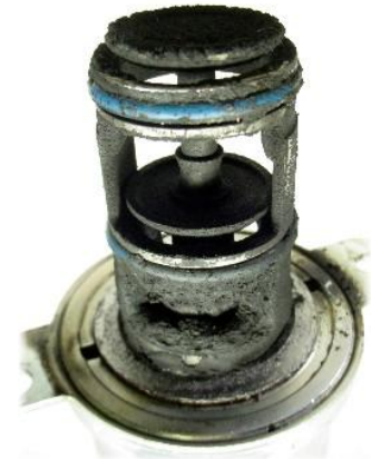
Figure 1: Failed EGR Valve due to particulate contamination
